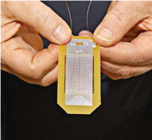
Industrial production would not be possible at this stage: First the 3.6 meter-long wire is etched into the ultra-thin aluminum membrane, and then the waffle pattern is embossed.
